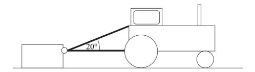
When the tractor moves forward, the crate accelerates at  $0.3\,\mathrm{m\,s^{-2}}$ . The coefficient of friction between the crate and the surface is 0.4.
